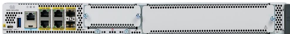
Figure 3. C8300-1N1S-4T2X is a 1RU platform with 1 SM slot and 1 NIM slot plus 2 x 10Gbps and 4 x 1Gbps embedded Layer3 Ethernet ports
