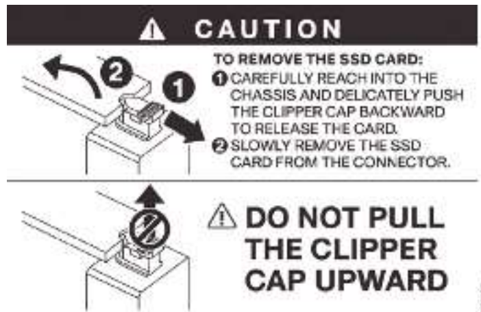
Figure 9: SSD Card Removal Instructions
