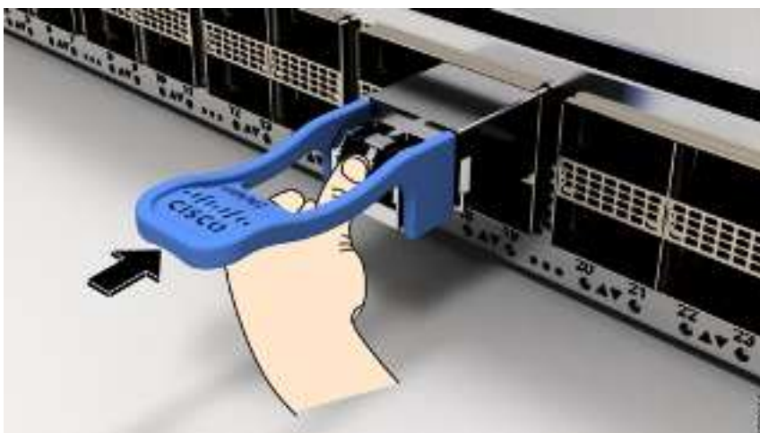
Figure 63: Seating the QSFP Transceiver Module
