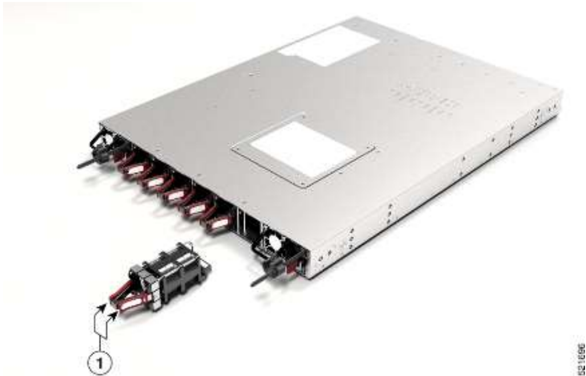
Figure 68: Cisco 8201-32FH and Cisco 8201-24H8FH Routers — Remove Fans
