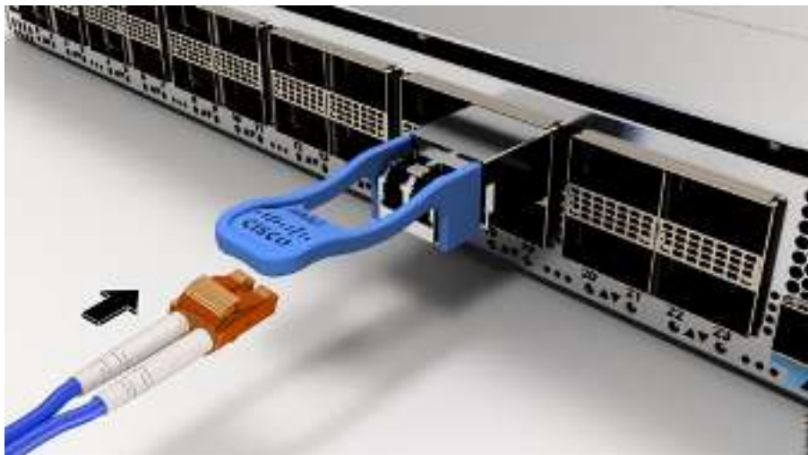
Figure 64: Cabling a Transceiver Module
