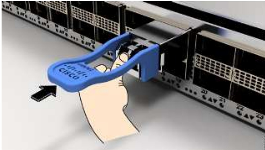
Figure 98: Seating the QSFP Transceiver Module
