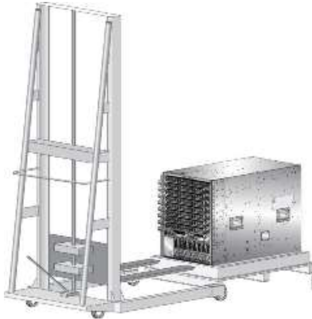
Figure 12: Align the Lifting Device in Front of the Chassis on the Pallet
