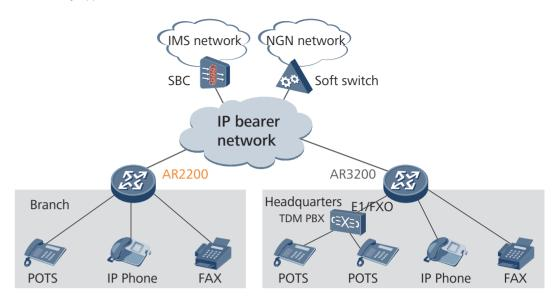
The AR2200 integrates voice, fax, and IP services. For enterprise users, the AR2200 serves as the SIP access gateway for a branch office, transforming phone signals into VoIP signals. The AR2200 uplink interfaces connect to the IP Multimedia Subsystem (IMS) or Next Generation Network (NGN) to allow any media, including phones, handsets, and computers to communicate at any time.
