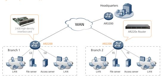
For investment protection, the AR2200 features a highly modular design. In the example above, a high-density GE access interface card is deployed to provide Gigabit speed access at a branch office.
